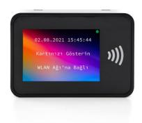
MCR04-W is a programmable 13.56MHz RFID Card Reader&Communication Terminal Device with Wi-Fi/Bluetooth connectivity, color TFT screen and high security protocols (such as HTTPS, MQTTS, TLS/SSL) supportability which can be used in Access Control, Personnel Attendance Control Systems, Closed-Loop Payment Systems, Telemetry&IoT applications etc.
