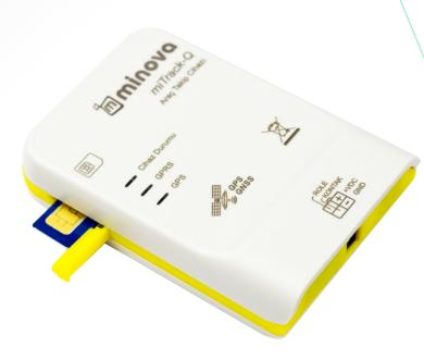
miTrack-Q, is a GPRS/2G/GNSS based tracking terminal. Installation is easy and fast with internal GSM and GPS antennas. Battery option which provides generate an alarm against dismantled is available. Measuring driving dynamics and severity (aggressive acceleration, sudden brakes, hard turns, etc.) is possible through standard Motion Sensor. Input/Output ports for contact detection and motor blockage are available as standard.
